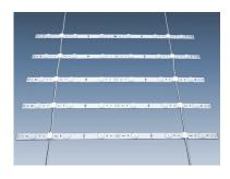
LED lattice light for backlighting large areas or displays. Light consisting of 27I LED bars connected parallel in a distance of 75 mm. Each LED bar is fitted with 6 high-power LEDs with front lens. Each bar 4.2 W and approx. 400 lm., dimensions 496 x 18 x 7 mm
