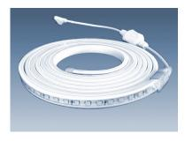
LED strip in robust, flexible plastic shell, 8.5 W/m, 72 LED/m, dimmable, width 17 mm, length 50 m, cuttable every 100 cm. Power supply by 230 V (no transformer required)
