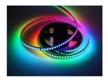
Flexible LED strip, equipped with individually addressable RGB LEDs, 43.2 W/m max., 144 LEDs/m, width 12 mm, length 2 m (one reel), dimmable, cutable at each LED, self-adhesive.
