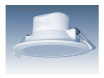
Powerful, completely encapsulated LED downlight 14 W, in robust plastic housing, with front glass and integrated power supply. Color temperature (CCT) adjustable by slide switch from coolwhite (approx. 6000 K), over neutralwhite (approx. 4000 K), to warmwhite (approx. 3000 K)
