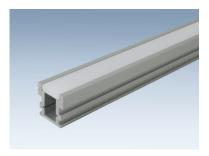
Walkable aluminium profile for floor mounting, with diffusor, with end caps. Suitable for led strips up to 11 mm width. Usuable in dry indoor areas. Loadable up to 10 kN
