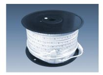
RGB LED strip in robust, flexible plastic shell, 8 W/m, 60 LED/m, dimmable, width 15 mm, length 50 m, cuttable every 100 cm. Power supply by 230 V (no transformer required). Incl. RGB controller (without remote)
