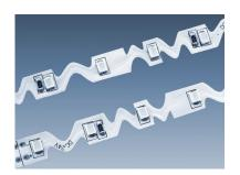
Highly flexible and bendable RGB LED strip (LED zigzag strip), installable in almost any shape. 12 W/m, 60 LEDs/m, width 8 mm, length 5 m (one reel), dimmable, every 12.5 cm cutable,
