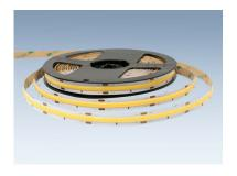
Flexible LED strip, equipped with seamless COB LEDs (528 chips/m), creating an uniform light band without any visible LED dots (totally dot-free), beam angle 180°, CRI > 90, self-adhesive, width 10 mm, dimmable, length 5 m, cuttable each 45 mm
