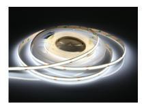
Flexible LED strip, equipped with seamless COB LEDs (480 chips/m), creating an uniform light band without any visible LED dots (totally dot-free), beam angle 180°, CRI > 90, self-adhesive, width 8 mm, dimmable, length 5 m, cuttable each 50 mm
