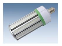
Powerful LED light, dimmable by remote, for backlighting very large three-dimensional forms, like picture cubes and light pillars. Equipped with 504 LEDs, covered by protective glass. Power supply by 100-240 V, no external driver needed. Socket E40. Passive cooling (no fan)
