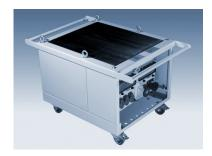
Mobile/movable isolating transformer for use on building sites, in tank construction, in the workshop among others. Robust metal housing, IP54, on castors, with transport lugs. Input 3 x 400 V with 16 A-CEE plug. 3 outputs 230 V with 16 A Schuko socket (continuous nominal power 14.5 A each). Secondary automatic circuit breaker for each socket with different power)
